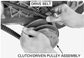
Remove the clutch/driven pulley assembly from the drive belt by holding the movable driven face.
