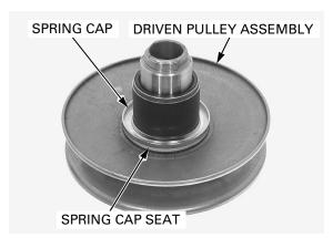
Install the driven face spring and spring seat.
