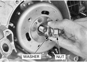
Hold the flywheel with the special tool and tighten the nut to the specified torque.
