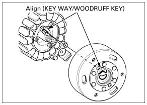
Install the washer and flywheel nut.
