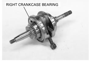
If the timing sprocket teeth are worn or damaged, check the cam chain, tensioner and cam sprocket.
