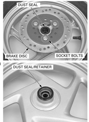
Remove the dust seal/retainer from the right wheel hub.
