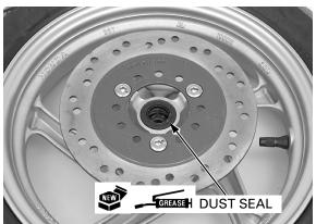
Install a new dust seal/retainer into the right wheel hub until it is fully seated.
