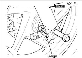
Install the axle nut and tighten it to the specified torque.
