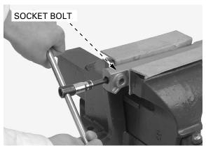
Remove the fork cap bolt and O-ring.
