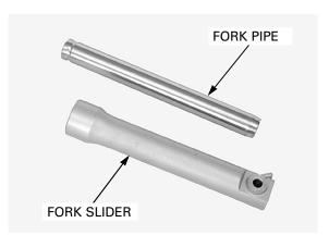
Set the fork pipe in V-block and measure the runout with a dial gauge.
