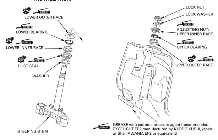
Install the washer to the steering stem.
