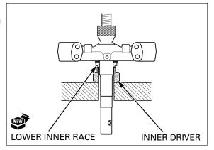
Install a new dust seal to the lower inner race groove.
