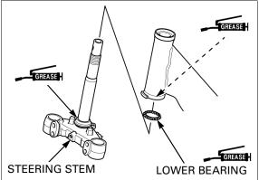
Apply each 3 – 5 g of grease with extreme pressure agent (recommended: EXCELIGHT EP2 manufactured by KYODO YUSHI, japan or Shell ALVANIA EP2 or equivalent) to upper inner race, upper bearing and upper outer race.
