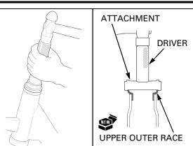
Drive a new lower outer race into the head pipe using the following tools.
