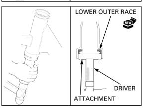
Apply each 3 – 5 g of grease with extreme pressure agent (recommended: EXCELIGHT EP2 manufactured by KYODO YUSHI, japan or Shell ALVANIA EP2 or equivalent) to lower inner race, lower bearing and lower outer race.
