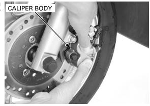
Remove the brake pad pin plugs. Loosen the brake pad pins.
