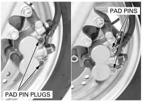
Remove the mounting bolts and remove the brake caliper from the brake disc.
