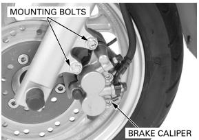
Remove the pad pins and brake pads.
