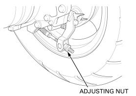
Loosen the lock nut and turn the adjuster until the play of the connecting cable becomes maximum.
