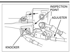
Check that there is no gap between the knocker pin and the end of the slot of the knocker joint.
