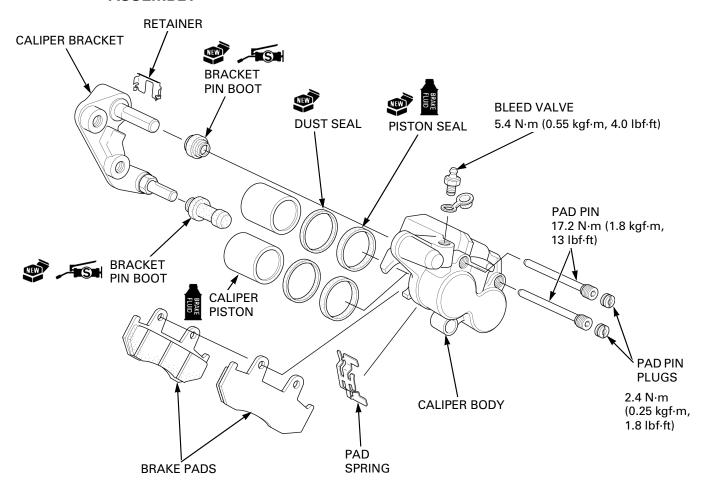
Coat new piston seals with DOT 3 or DOT 4 brake fluid.
