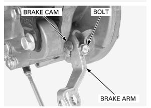
Remove the brake cam from the brake panel.
