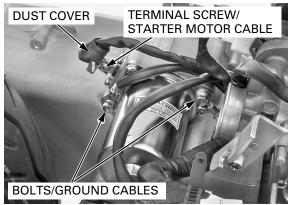
Remove the starter motor from the left crankcase. Remove the O-ring from the starter motor.
